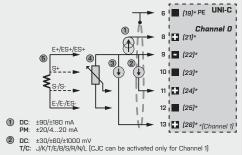
±20/±40/±80 V ±2/±5/±10 V DU: Linear potentiometer (min. 500 Ω)
