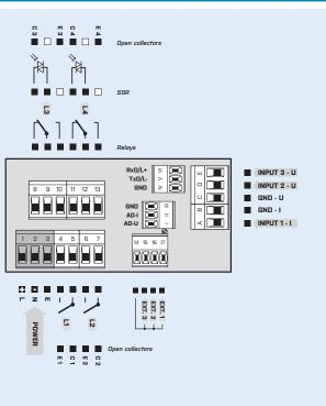
\* GND (input) is galvanically connected with inputs EXT. and the OM Link connector
