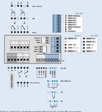
\*GND (input + Option A) is galvanically connected with inputs EXT. and the OM Link connector \*In case of Option B we recommend to connect termianls GND (main board/additional board) by external connection
