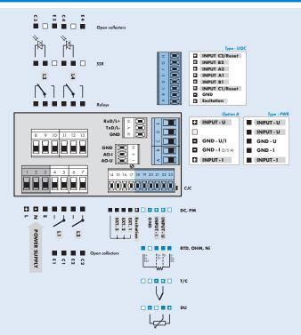
\*GND (input + Option A) is galvanically connected with inputs EXT, and the OM Link connector \*In case of Option B we recommend to connect termianIs GND (main board/additional board) by external connection
