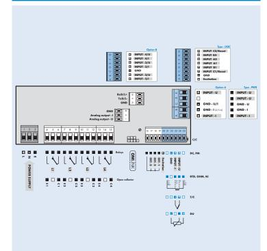
\*GND (input + Option A) is galvanically connected with inputs EXT. and the OM Link connector \*In case of Option B we recommend to connect termianls GND (main board/additional board) by external connection
