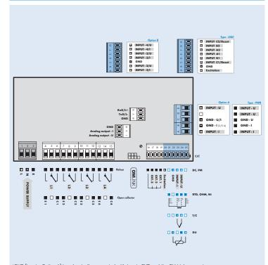
\*GND (input + Option A) is galvanically connected with inputs EXT. and the OM Link connector \*In case of Option B we recommend to connect termianIs GND (main board/additional board) by external connection
