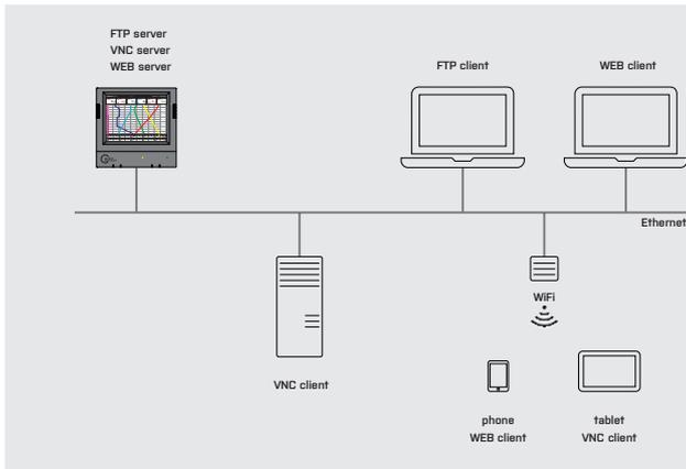
In its basic version the recorder is equipped with connection Ethernet 10/100Base and offers:
