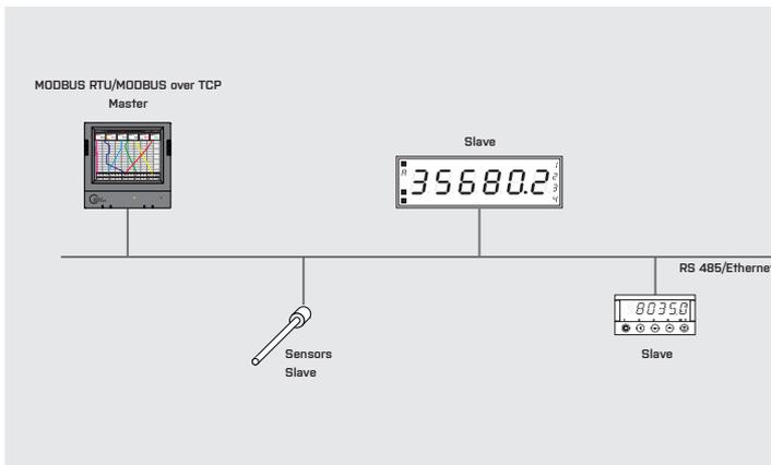
Under preparation is the second version, offering use of data line RS485 with a MODBUS RTU protocol. Up to 247 devices can be connected to the line.
