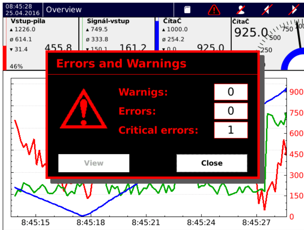
Errors and warnings window showing one detected critical error.
