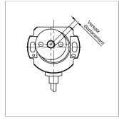
Lateral magnet offset will cause additional linearity error. The angle error, which is caused by radial displacement of sensor and position marker depends on the used position marker or magnet.
