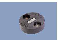
The sensor utilizes the orientation of a magnetic field for the determination of the measurement angle. Therefore, a position marker is attached to the rotating shaft. The magnetic field orientation is captured with an integrated circuit. An analogue output signal represents the calculated angle.
