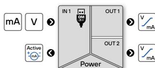
The OMX 200 model series are digital DIN rail mounted signal converters housed in an enclosure only 12.5 mm wide.
